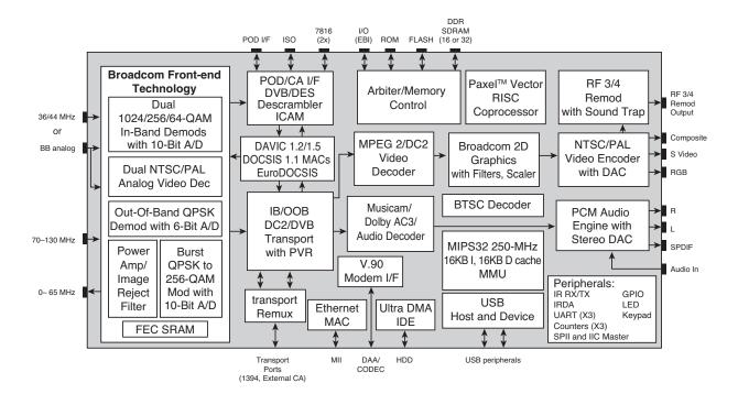
The **BCM7110** is a single-chip set-top box device that combines the key aspects required for the next generation of set-top boxes including cost-effective single-chip design, personal video recording (PVR), broadband communication via DOCSIS™ 1.1 cable modem, and support of all major global standards for worldwide deployment.
