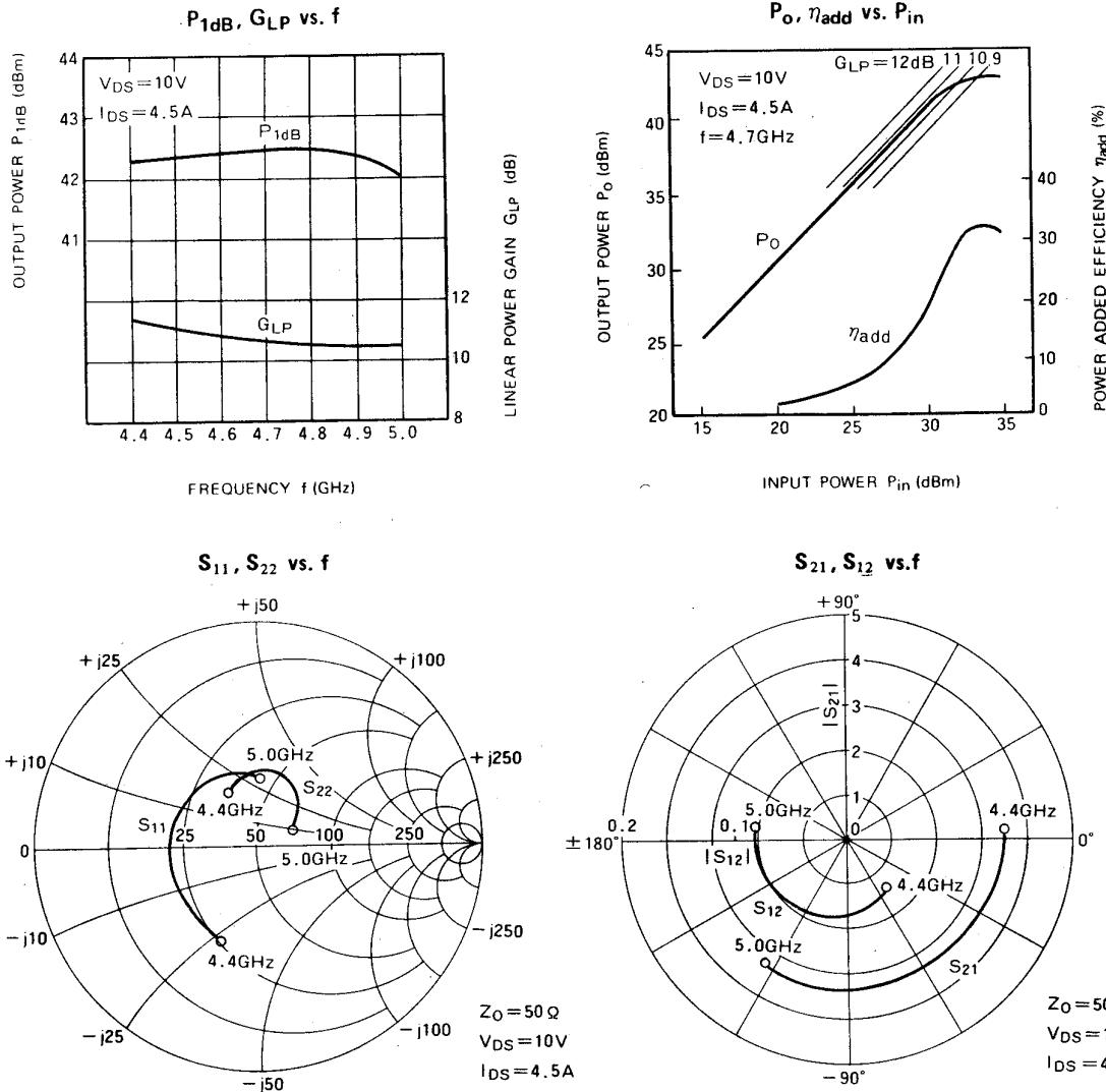
**S PARAMETERS ( $T_a = 25^\circ C$ ,  $V_{DS} = 10V$ ,  $I_{DS} = 4.5A$ )**
