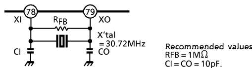
Fig.1(a) Self excited crystal oscillator
