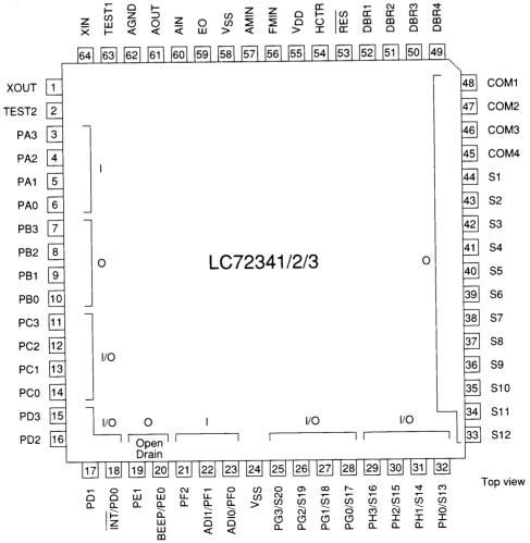
\* PE0 and PE1 are open-drain outputs.
