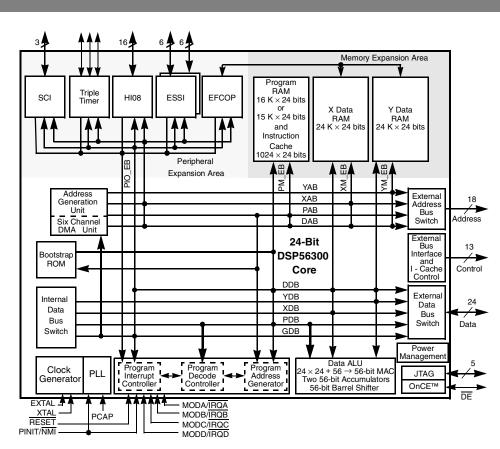
Figure 1. DSP56L307 Block Diagram
