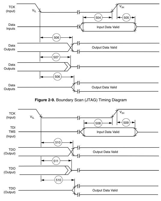
Figure 2-10. Test Access Port Timing Diagram
