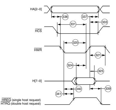
Figure 2-26. Write Timing Diagram, Non-Multiplexed Bus, Double Data Strobe
