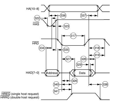
Figure 2-28. Read Timing Diagram, Multiplexed Bus, Double Data Strobe
