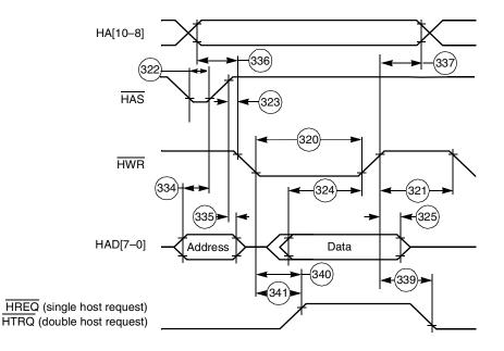
Figure 2-30. Write Timing Diagram, Multiplexed Bus, Double Data Strobe
