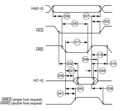
Figure 2-24. Read Timing Diagram, Non-Multiplexed Bus, Double Data Strobe
