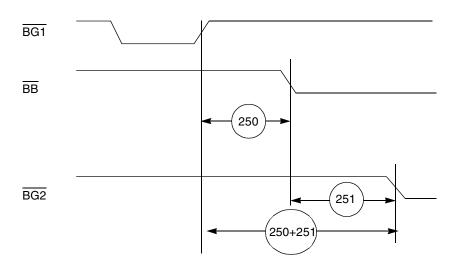
Figure 2-21. Asynchronous Bus Arbitration Timing
