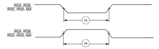
Figure 2-5. External Interrupt Timing (Negative Edge-Triggered)
