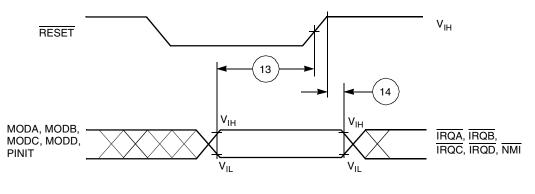
Figure 2-6. Operating Mode Select Timing
