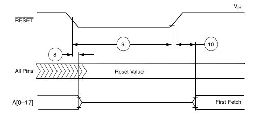
Figure 2-3. Reset Timing
