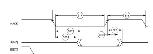
Figure 2-22. Host Interrupt Vector Register (IVR) Read Timing Diagram
