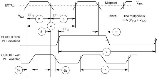
Figure 2-2. External Clock Timing
