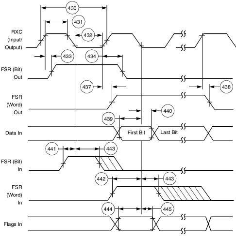
Figure 2-2. ESSI Receiver Timing
