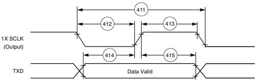
Figure 2-32. SCI Asynchronous Mode Timing
