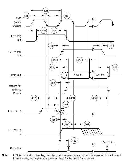
Figure 2-1. ESSI Transmitter Timing
