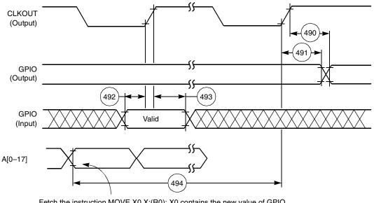
Fetch the instruction MOVE X0,X:(R0); X0 contains the new value of GPIO and R0 contains the address of the GPIO data register.
