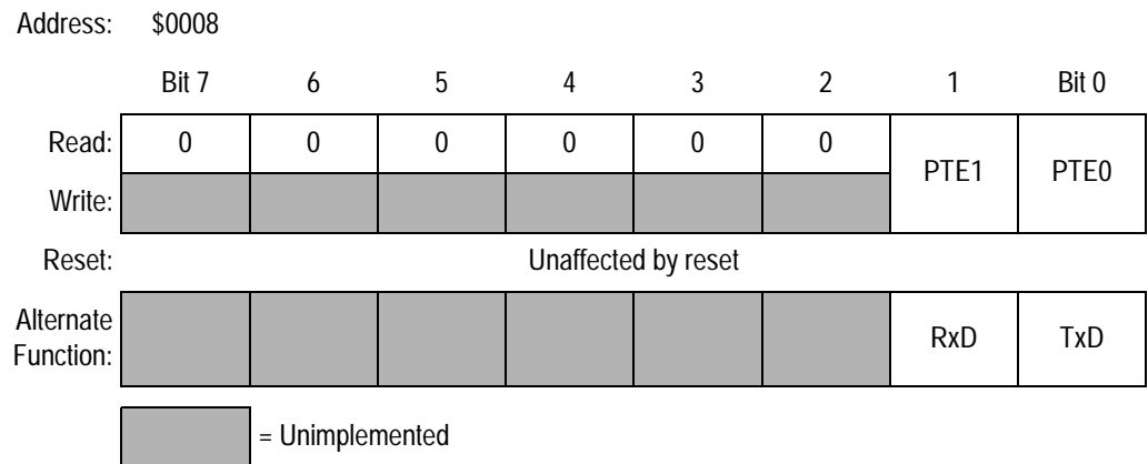
Figure 16-17. Port E Data Register (PTE)
