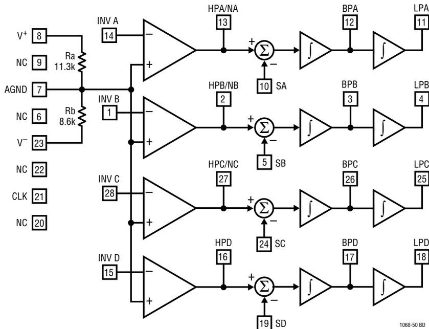
NOTE: THE RATIO OF  $R_a/R_b$  CAN VARY BY  $\pm 0.8\%$ .
