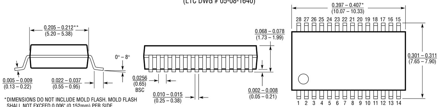
\* DIMENSIONS DO NOT INCLUDE MOLD FLASH. MOLD FLASH SHALL NOT EXCEED 0.006" (0.152mm) PER SIDE
