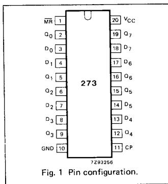
Fig. 1 Pin configuration.
