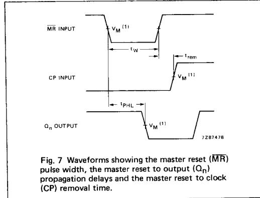
Fig. 7 Waveforms showing the master reset (MR) pulse width, the master reset to output ( $Q_n$ ) propagation delays and the master reset to clock (CP) removal time.
