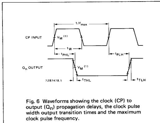
Fig. 6 Waveforms showing the clock (CP) to output ( $Q_n$ ) propagation delays, the clock pulse width output transition times and the maximum clock pulse frequency.
