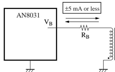
$R_B$  too large: Consumption current becomes small, however,  $T_{OFF}$  is extended by the delay amount because of low speed.
