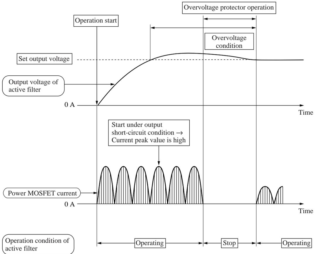
Figure 12. Output voltage overshoot when operation starts
