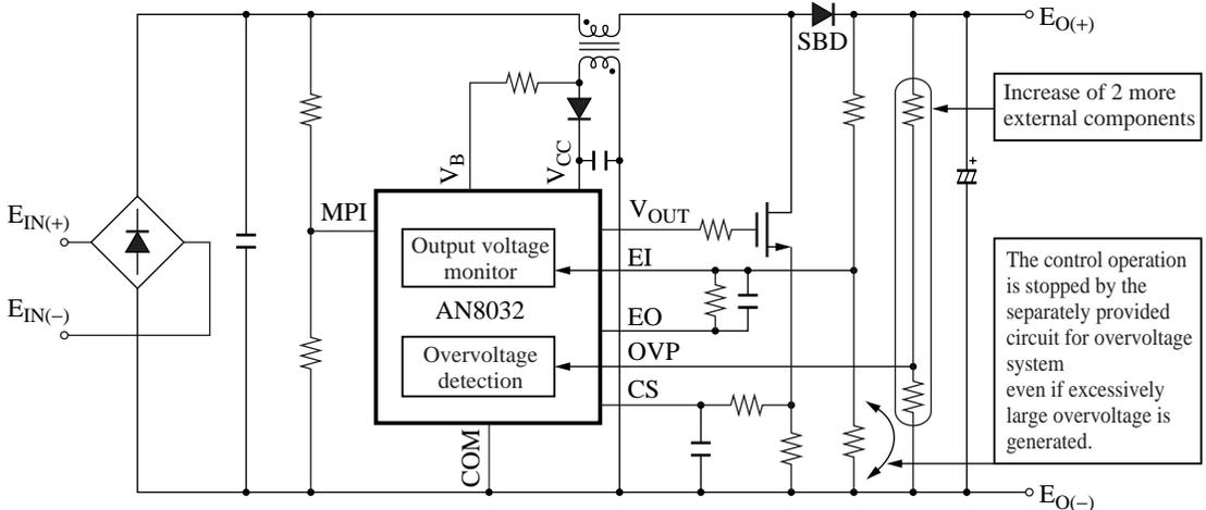
Note) The OVP terminal is arranged beside the EI terminal after taking the board pattern design into consideration.
