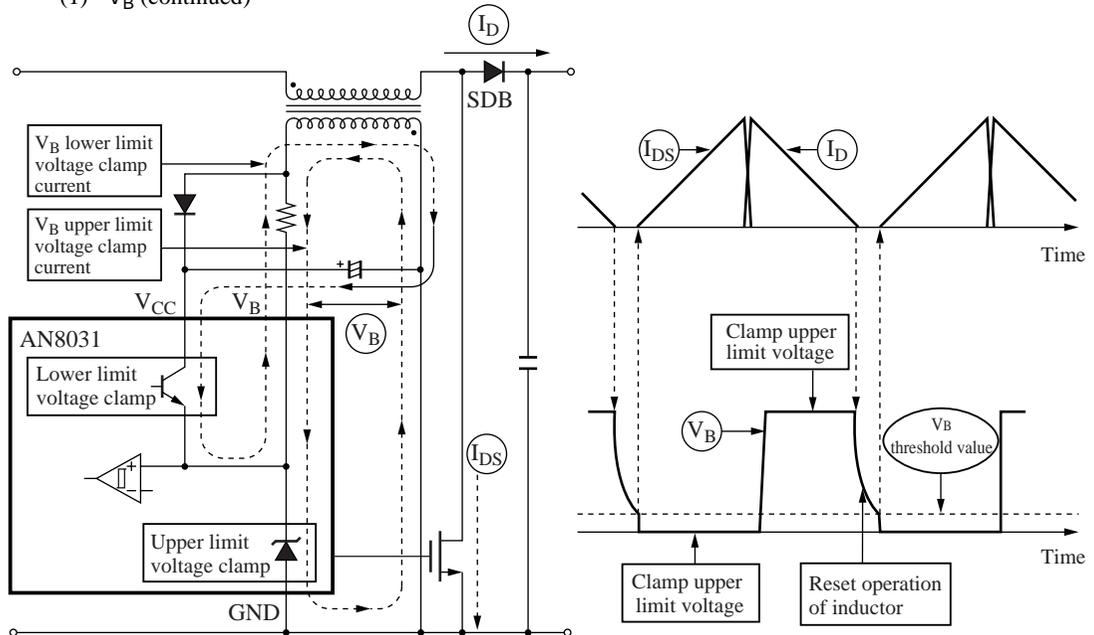
Figure 5. Explanation of  $V_B$  operation
