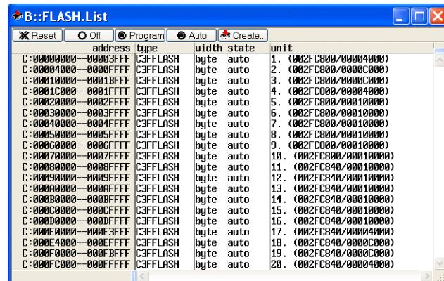
The NEXUS debugger supports the programming of external flash memory as well as the programming of internal flash memory of microcontrollers. The
