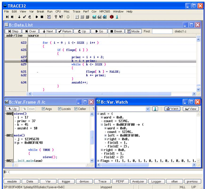
A hierarchical symbol database enables structured symbolic debugging. Symbol names can be used to show single program addresses, mod-
