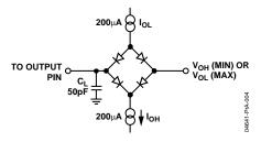
Figure 5. Load Circuit for SDO Timing Diagram
