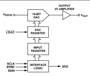
Figure 9. Simplified Serial Interface showing input loading circuitry for one DAC Channel
