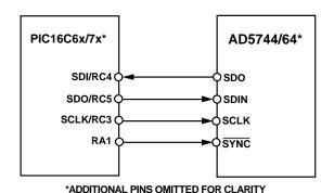
Figure 15. AD5744/64 to PIC16C6x/7x Interface
