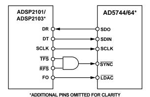
Figure 14. AD5744/64 to ADSP2101/ADSP2103 Interface
