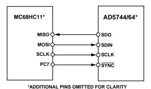
Figure 13. AD5744/64 to MC68HC11 Interface
