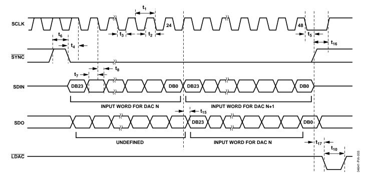
Figure 3. Daisy Chain Timing Diagram
