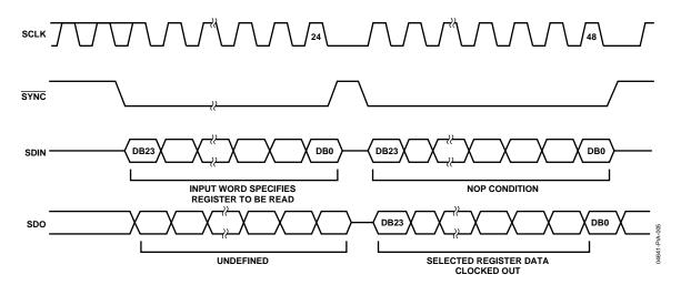
Figure 4. Readback Timing Diagram
