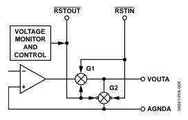
Figure 10. Analog Output Control Circuitry
