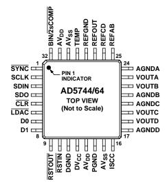
Figure 6. 32-Lead TQFP Pin Configuration Diagram
