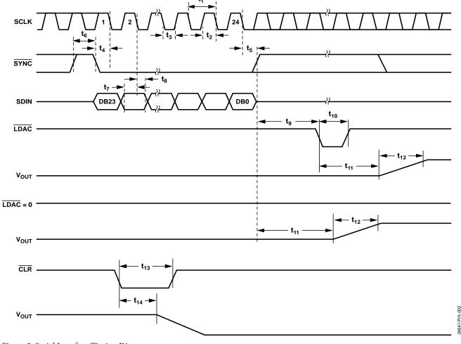
Figure 2. Serial Interface Timing Diagram
