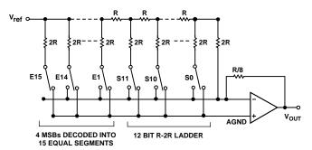
Figure 7. DAC Ladder Structure
