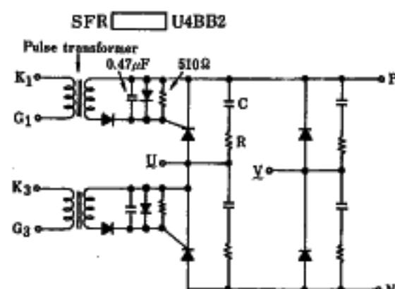
The stack with fuse is coded to the SFR [ ] [ ] 4BB3 series.
