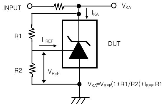
Fig. 3 Test Circuit for  $I_{KA}$  (off)
