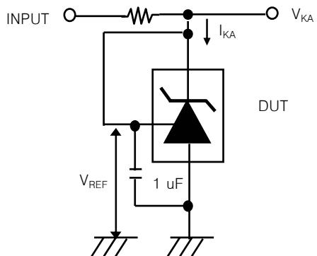
Fig. 2 Test Circuit for  $V_{KA} \geq V_{REF}$
