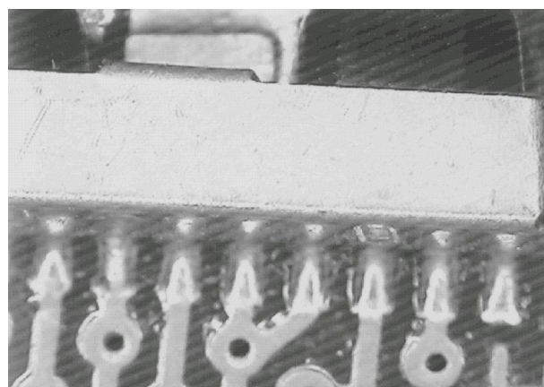
Photo 4.0. Unit self-aligns after reflow.
