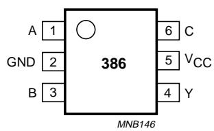
Fig.1 Pin configuration.
