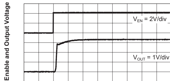
Turn-On Time From Enable ( V_{IN} = 4.2\text{V} ; I_{OUT} = 300\text{mA} )
