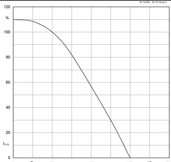
Fig. 2 : Rated forward current vs. ambient temperature
