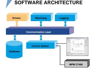
U9046 consists of several software components to perform the measurement in real time with great flexibility.
