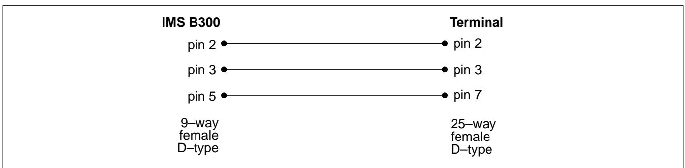
Figure 1 Example cable connection to diagnostic terminal
