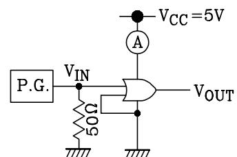
Input waveform is the same as that in case of switching characteristics test.
