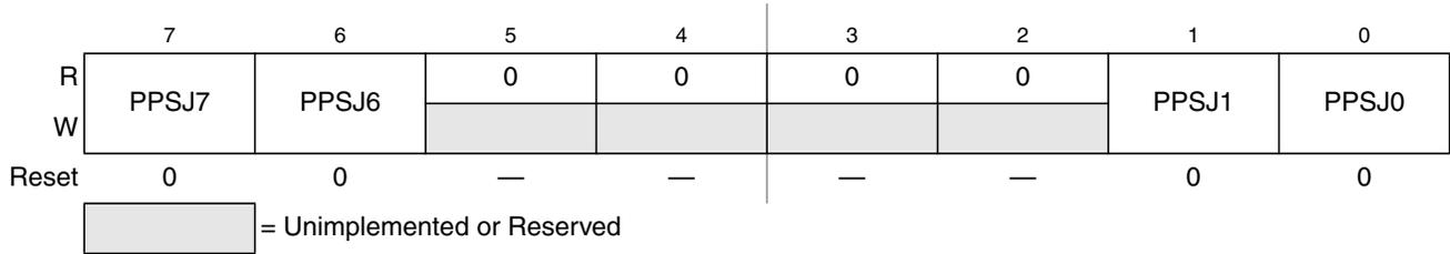
**Figure 2-45. Port J Polarity Select Register (PPSJ)**
