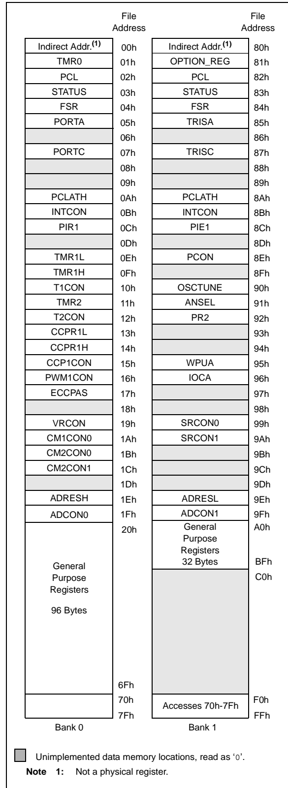
FIGURE 2-4: DATA MEMORY MAP OF THE PIC16F616/16HV616
