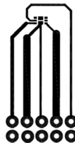
b. 182^\circ\text{C}/\text{W} when mounted on a minimum pad of 2 oz copper
