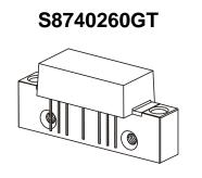
GaAs Push Pull Hybrid 40 – 870MHz 26.0dB min. Gain @ 870MHz 240mA max. @ 24VDC
