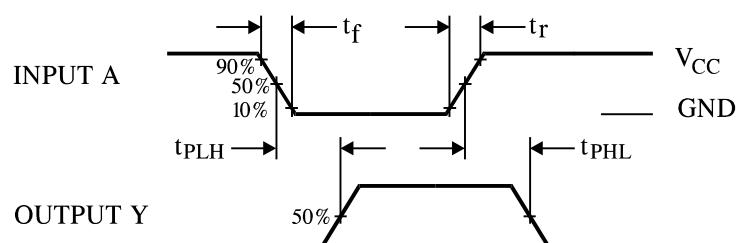
**Figure 1. Switching Waveforms**
