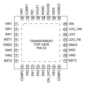
Figure 3. 34700 Pin Connections
