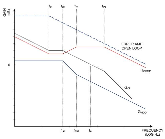
Figure 12. Bode Plot of the Buck Converter
