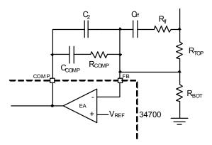
Figure 11. Type III Compensation Network
