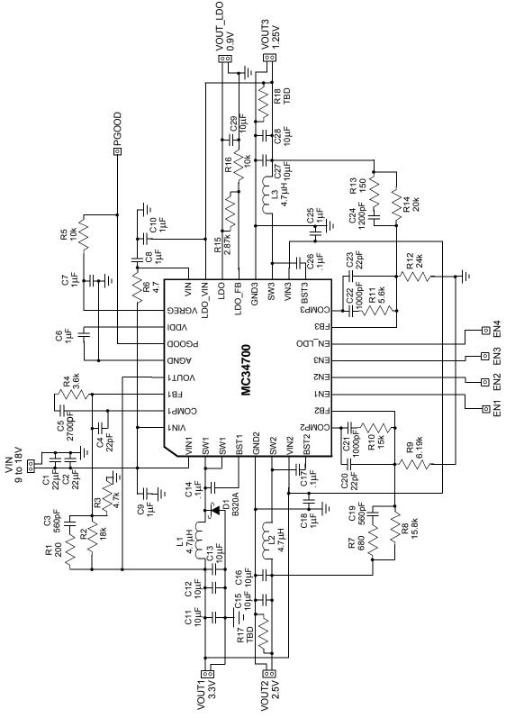
**Figure 5. Typical Application Diagram**
