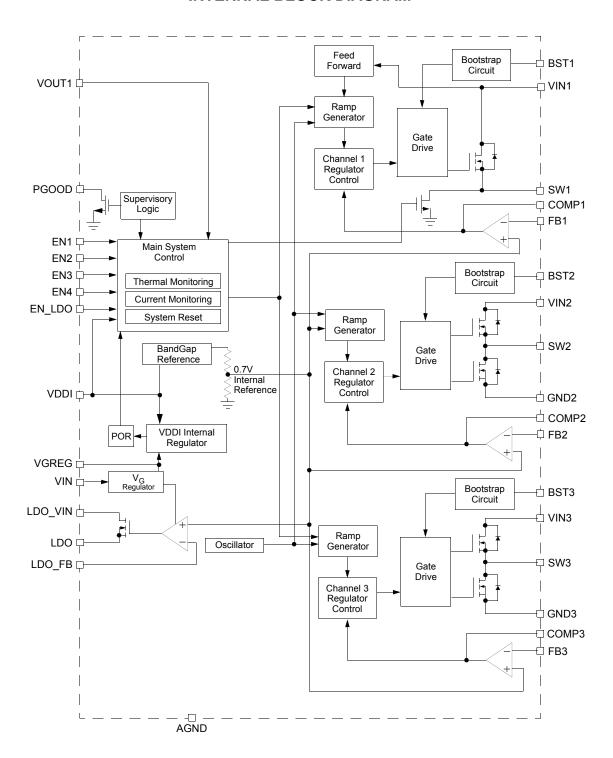
Figure 2. 34700 Simplified Internal Block Diagram
