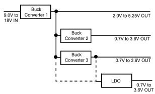
Figure 8. Single Input Supply Configuration
