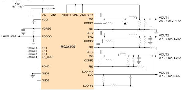
Figure 1. MC34700 Simplified Application Diagram
