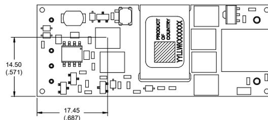
EUE120: SO-8 drain pin must not exceed 115°C.
