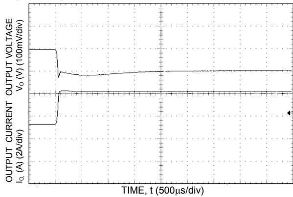
**Figure 13. Typical Transient Response to Step increase in Output Load from 5.3A to 8.1A at Room Temperature and 48 Vdc Input;  $C_{o,ext} = 370 \mu\text{F}$ .**
