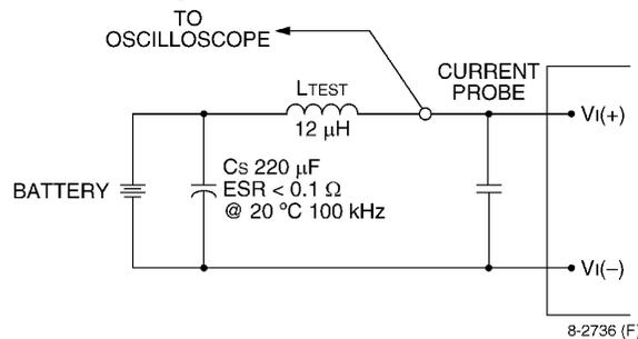
Note: Measure input reflected-ripple current with a simulated source inductance (LTEST) of 12 μH. Capacitor CS offsets possible battery impedance. Measure current as shown above.
