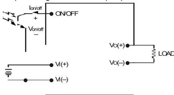
**Figure 20. Circuit configuration for using Remote On/Off Implementation.**
