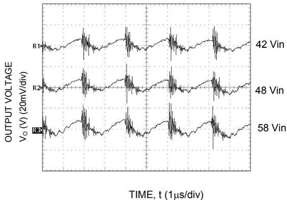
**Figure 11. Typical Output Ripple and Noise at Room Temperature and  $P_o = 120\text{W}$ .**
