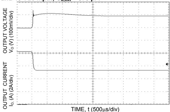
**Figure 14. Typical Transient Response to Step decrease in Output Load from 8.1A to 5.3A at Room Temperature and 48 Vdc Input;  $C_{o,ext} = 370 \mu\text{F}$ .**
