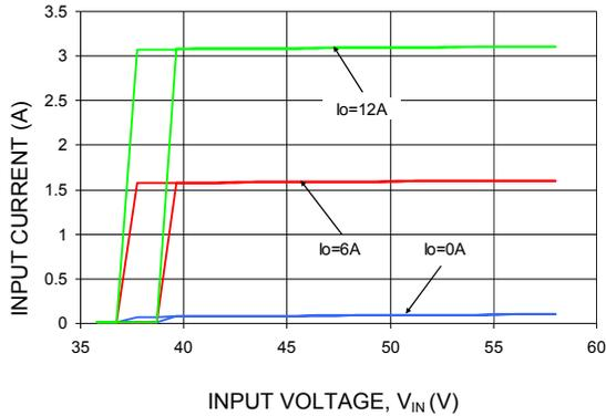
**Figure 9. Typical Input Characteristic at Room Temperature.**
