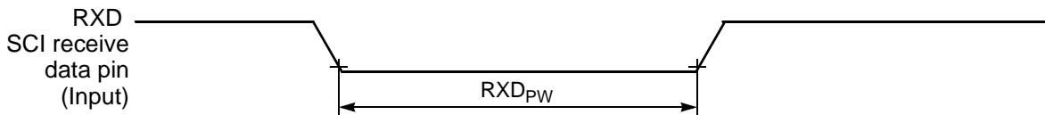
Figure 10-16 RXD Pulse Width
