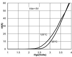
Figure 2: Transfer Characteristics
