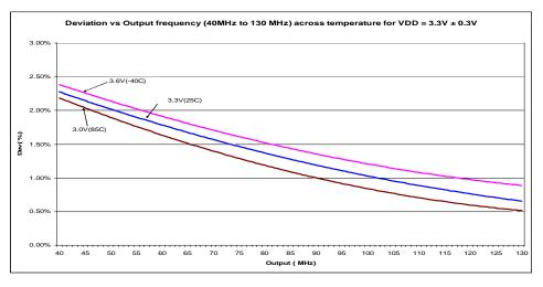
Note: Transition band is 30MHz to 34MHz for VDD= $2.5V \pm 5\%$ , across -40°C to +85C. Deviation in this band is  $1.93\% \pm 37\%$ . Transition band is 30MHz to 39MHz for VDD= $3.3V \pm 0.3V$ , across -40°C to +85C. Deviation in this band is  $1.8\% \pm 45\%$ .
