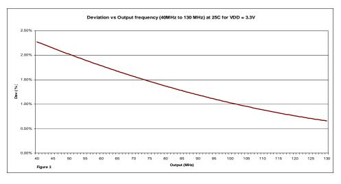
Note: Transition band is 30MHz to 34MHz for VDD=2.5V at 25°C. Deviation in this band is 2.5%  $\pm$  4%. Transition band is 30MHz to 39MHz for VDD=3.3V at 25°C. Deviation in this band is 1.8%  $\pm$  30%.
