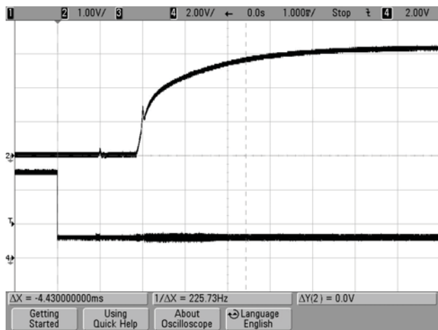
Enable Start-up ( V_{in}=48V I_{out}=20A )
