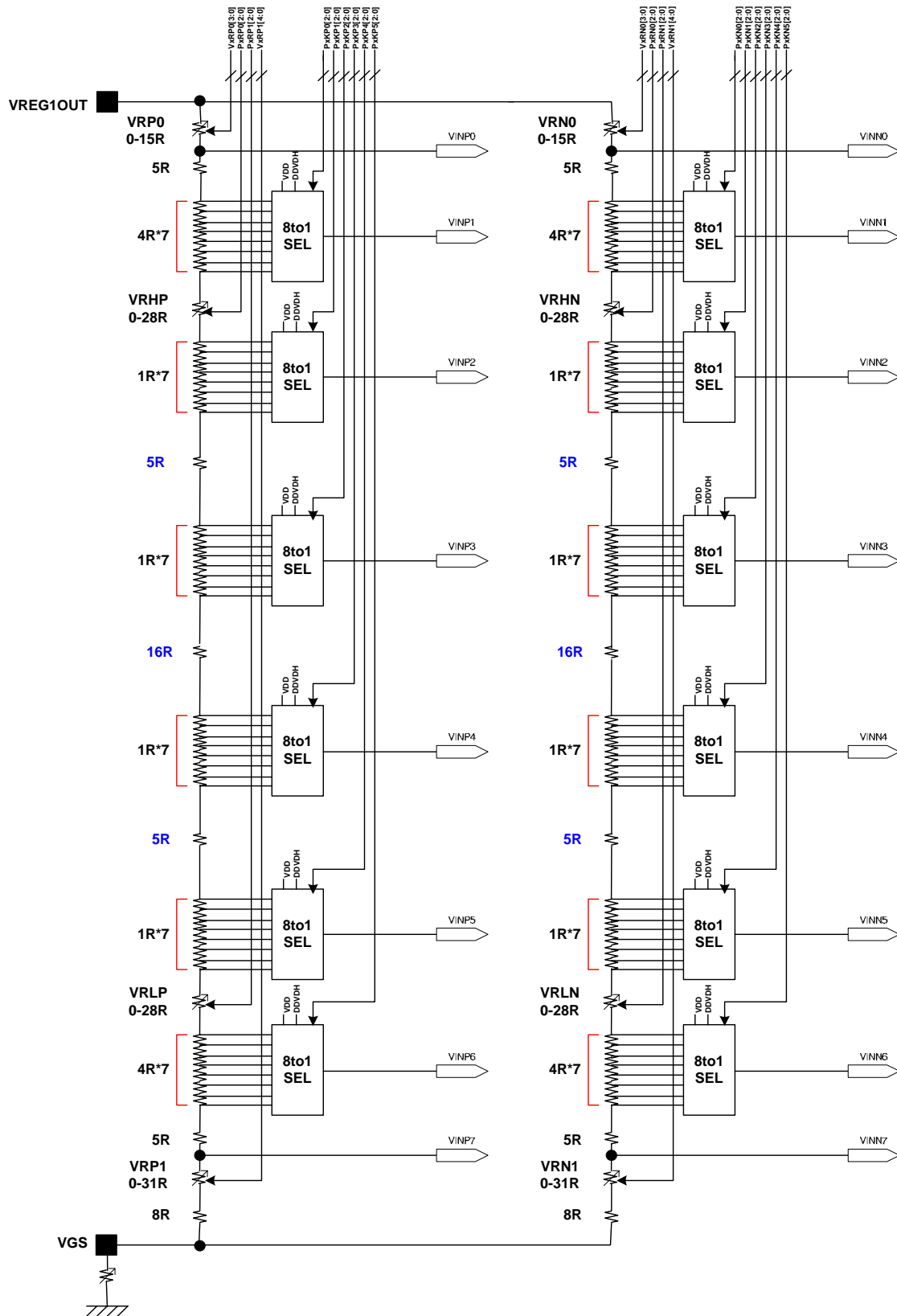
Figure 67 Ladder resistor units and 8-to-1 selectors (IPS=0)
