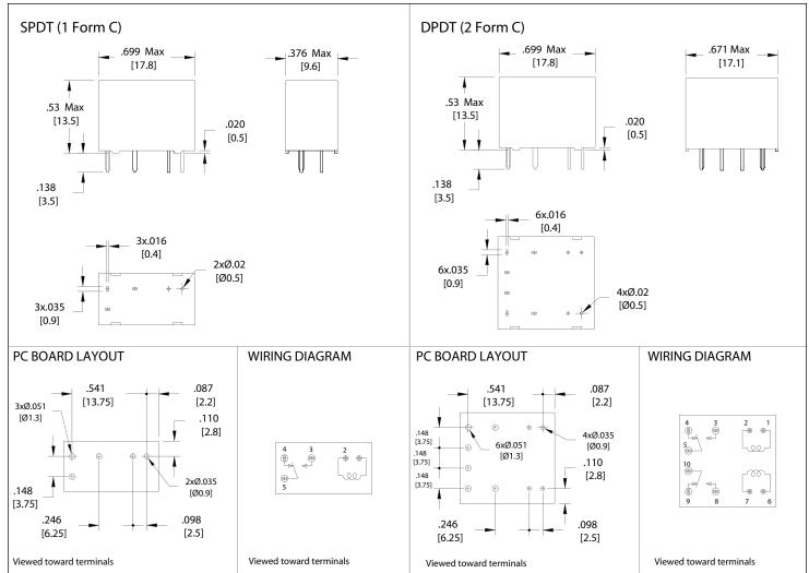
Dimensions in inches with metric equivalents in parentheses. Tolerance: ± 0.010"
