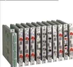
Install by inserting into the main unit. Can be replaced by user.
