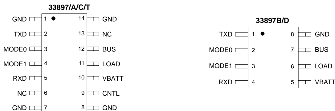
Figure 4. 33897/A/B/C/D/T Pin Connections
