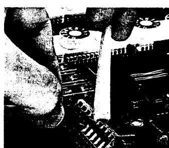
Connection of conductors with operating tool
