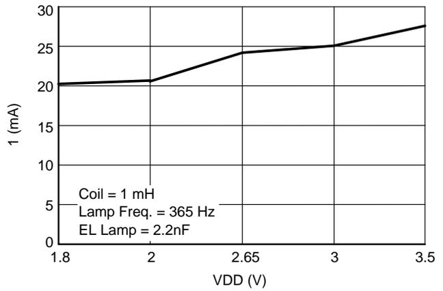
Figure 7. Current Consumption versus V<sub>DD</sub>
