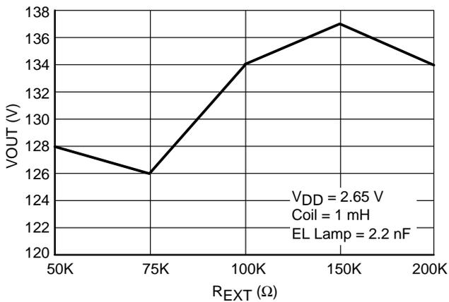
Figure 8. Output Voltage versus R<sub>EXT</sub>
