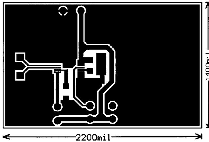
Figure 13. MC33441 PC Board – Bottom View
