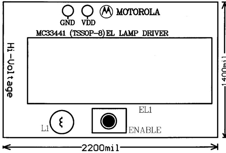
Figure 11. MC33441 PC Board – Top View
