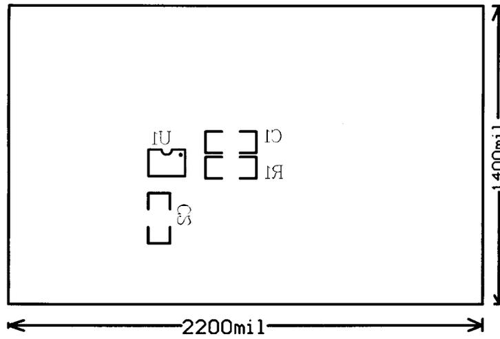
Figure 12. MC33441 Component Placement Guide – Component Side
