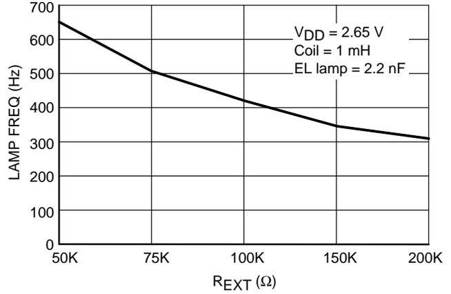
Figure 5. Lamp Frequency versus R<sub>EXT</sub>
