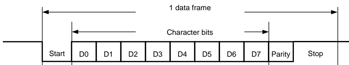
Figure 22-1. Data Format for Transmission and Reception
