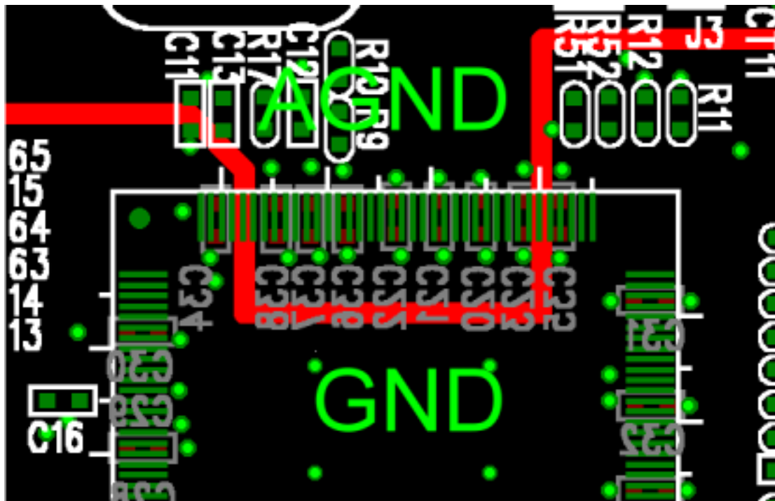
Figure 8. Reference Ground Partitions under the VT6202
