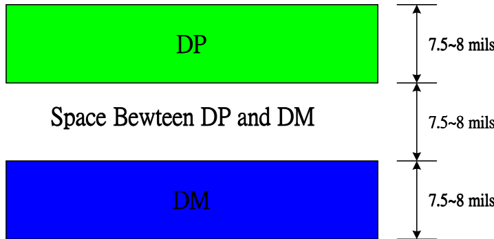
Figure 11. USB Differential Signal Routing
