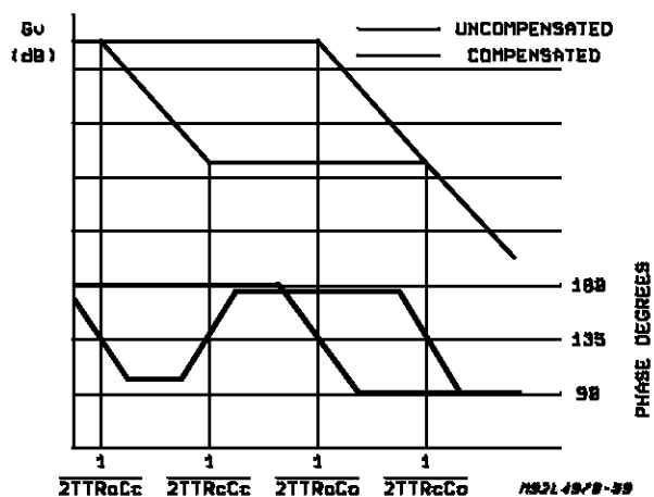
Figure 14: Bode plot showing gain and phase of compensated error amplifier.
