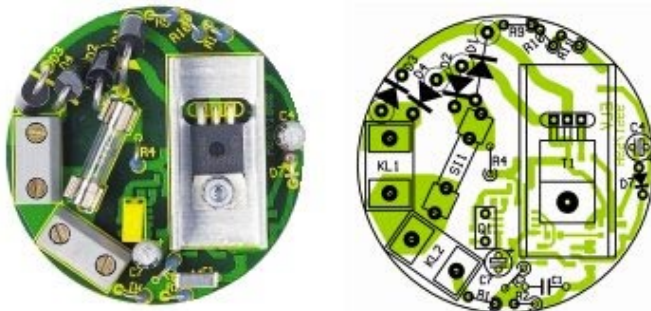
The fully assembled PCB for the DI 300, viewed from the component side, and the corresponding component mounting diagram
