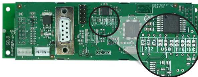
Figure 17: Protocol-Select-Jumpers for GLK19264-7T-1U Non-USB
