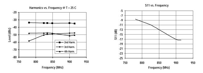
Test Conditions (Unless Otherwise Specified):  $V_{DD} = 5 V$ ,  $P_{IN} = +7 dBm$ ,  $V_{GG} = -3.5 V$ , Freq. = 824 & 849 MHz,  $T_c = 25^{\circ}C$ , Gate voltage determined by the recommended bias circuit
