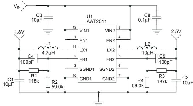
**Figure 1: AAT2511 Adjustable Output with Enhanced Transient Response.**
