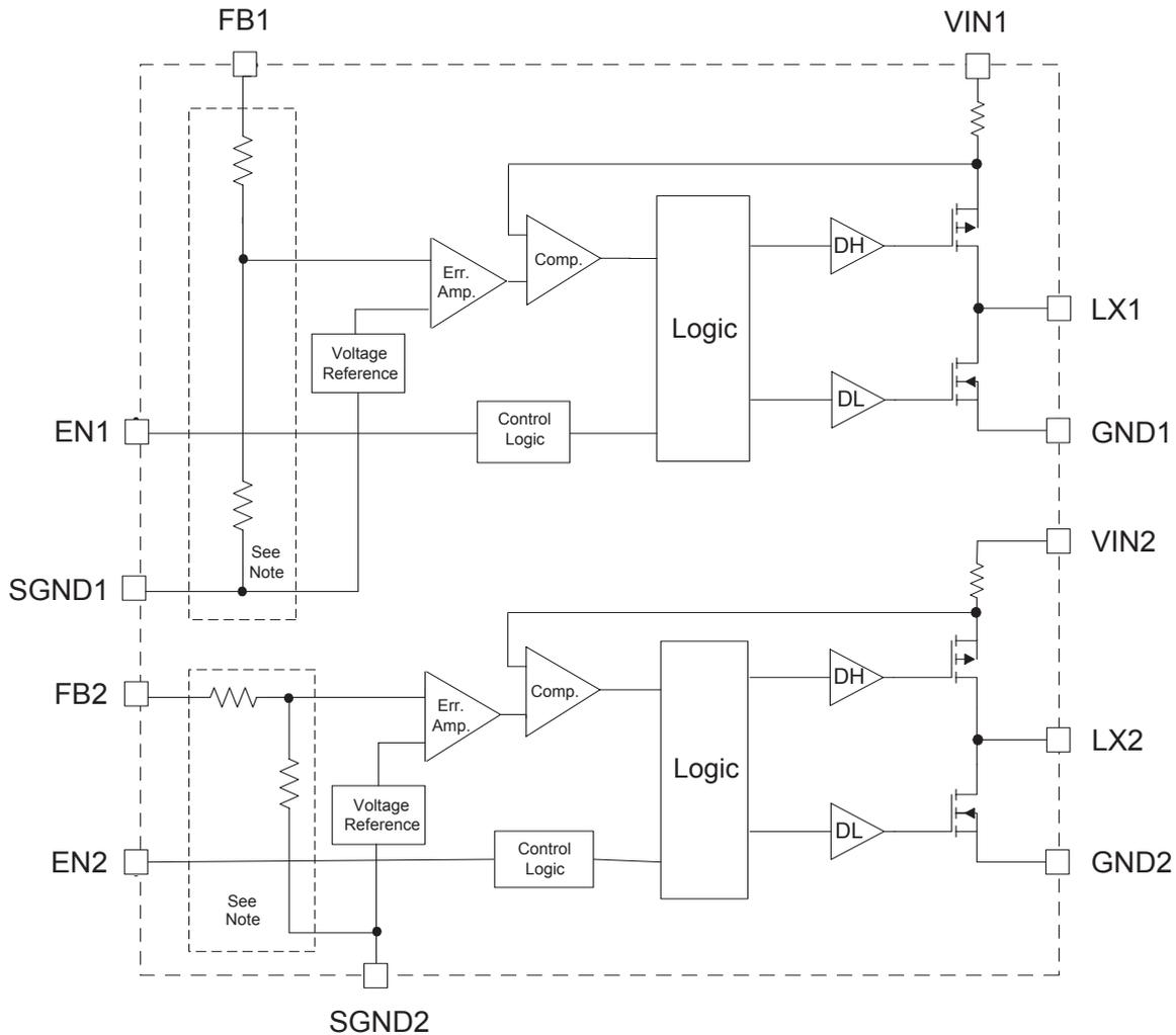
Note: Internal resistor divider included for  $\geq 1.2V$  versions. For low voltage versions, the feedback pin is tied directly to the error amplifier input.
