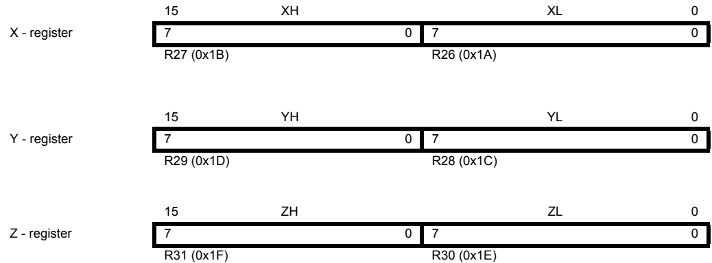
Figure 5. The X-, Y-, and Z-Registers
