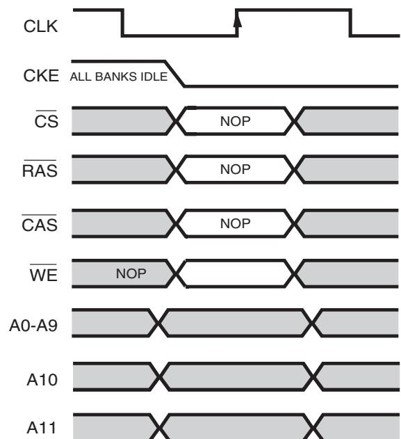
**Clock Suspend Command**
