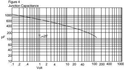
Junction Capacitance - pF *versus* Reverse Voltage - Volts
