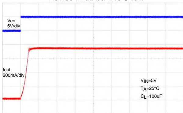
Short Circuit Current, Device Enabled Into Short
