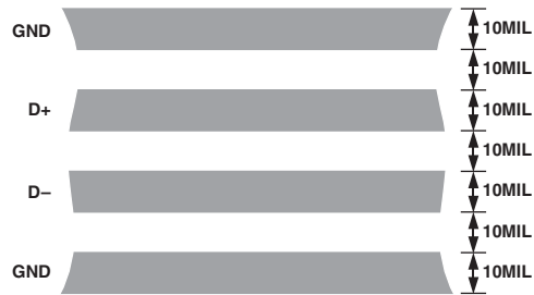
Figure 4. Arrangement of Signal Tracks
