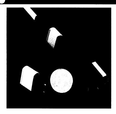
The MTP™ Multifiber Connector provides quick and reliable connection for up to 12 optical fibers in a compact housing. Two MT-style, push-on connectors are mated using a low-profile bulkhead or PC card-mounted adapter. Connection is assured by the spring-action side latch housing – simply push-on and pull-off. The MTP™ incorporates the Conec® MT-style Multifiber Ferrule. Evaluation cords and fan-outs with the MTP™ are available. Private label housing available.
